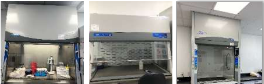
(From Left) Logic Biosafety Cabinet Class II-Type A2, Labconco Biosafety cabinet Class I and Labconco Echo Fume Hood
